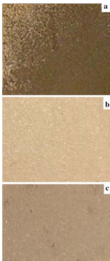
Fig. 4 Digital photos of the mild steel surface (a) after electrolyses with molybdate; (b) before any electrolyses; (c) after electrolyses with dichromate
